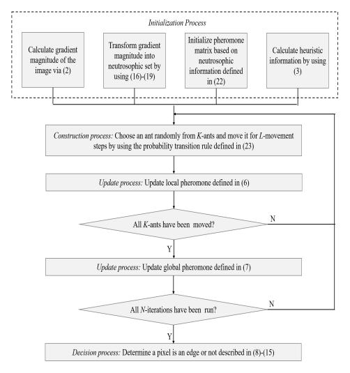
Figure 1. A summary of the implementation The Robust ACO Based On Neutrosphic Set of Gradient Magnitude
